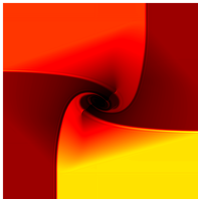
Figure: Four contact discontinuities 2D Riemann problem on a Cartesian mesh with 1.5 \times 10^6 DOF
