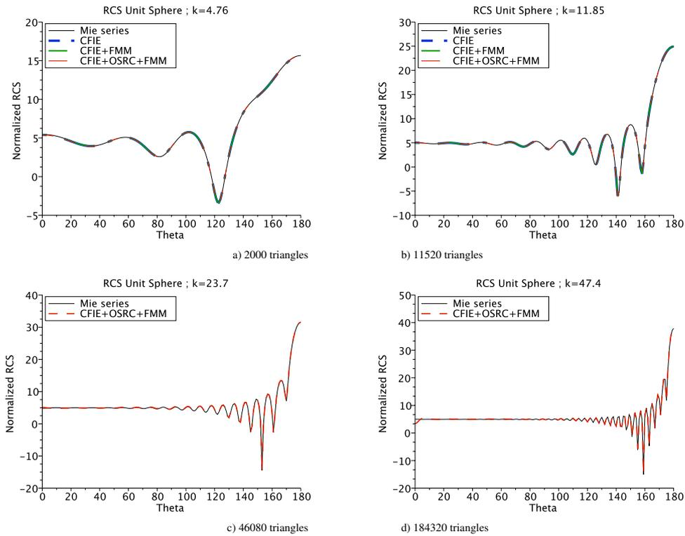
Figure 14: Scattering by a sphere (null incidence)
