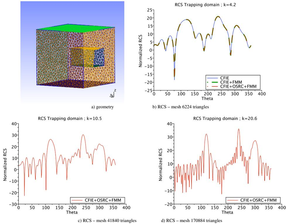
Figure 16: Scattering by a cube with reentrant structure, for  $\theta^{\text{inc}} = (\sqrt{3}/2, 0, 1/2)$
