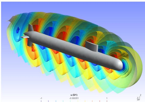
Figure 7: Scattering by a model submarine (by using a volumetric formulation, finite element methods, an artificial boundary condition and a domain decomposition algorithm).
