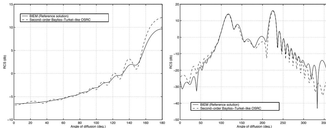
Figure 13: Computation of the bistatic RCS: Case 1: a plane wave of characteristics  $k = 14$  and  $\theta^{\text{inc}} = 0$  deg. illuminates the unit square cylinder for a Dirichlet boundary condition, Case 2: a plane wave of characteristics  $k = 20$  and  $\theta^{\text{inc}} = 45$  deg. illuminates a conesphere for a Neumann boundary condition.
